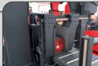
35- SERVO MOTOR FEEDING VICE 27" STROKE
