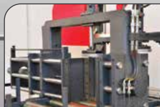
39- SERVO MOTOR FEEDING VICE 120" STROKE
