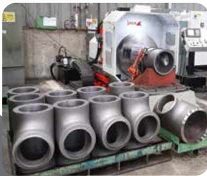
Complex Elbow Bevels Quickly Achieved
